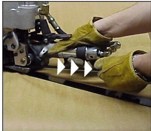
Pull back on the **TOP STRAP** to eliminate additional slack around the package. You will have to push on the cylinder cover to make certain that the jaw tips are in position over the seal.
