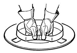
Lift upwards to free the liner from the base flange. Hold both ends of the liner firmly and lift the tab end to disengage the lock.
