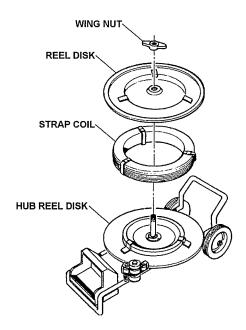
6. Position the three coil ties above the three small indentations. These indentations allow the ties to be removed without disturbing the coil.
