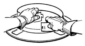
c. Allow the liner to slowly straighten before releasing either end.
