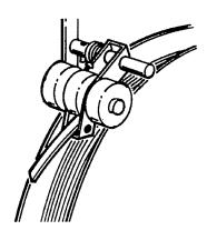
10. Replace and securely tighten the wing nut by turning it in the clockwise direction.
