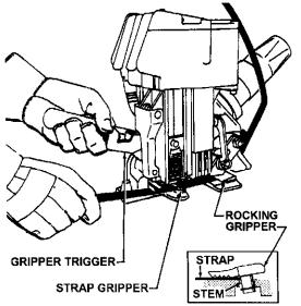
2. Insert the top strap between the feedwheel and the gripper plug and insert it into the slot of the strap latch. Pull excess slack from the strap. Make sure you are not standing in line with the strap and press the tensioner lever all the way down. It will lock in place. The feedwheel will engage automatically and the tool will begin tensioning. Should it become necessary to stop the tensioning cycle, press the valve latch forward.
